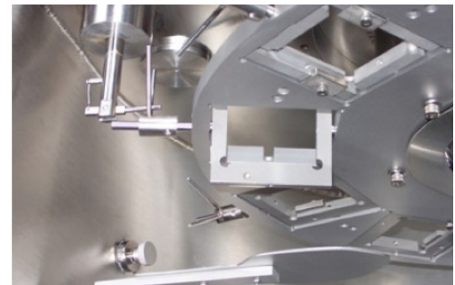
In Situ Flip Fixture Allows for Coating on Both Sides without Breaking Vacuum
