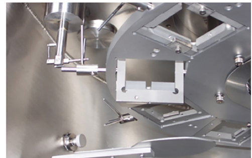
In Situ Flip Fixture Enables Coating Both Facets without Breaking Vacuum
