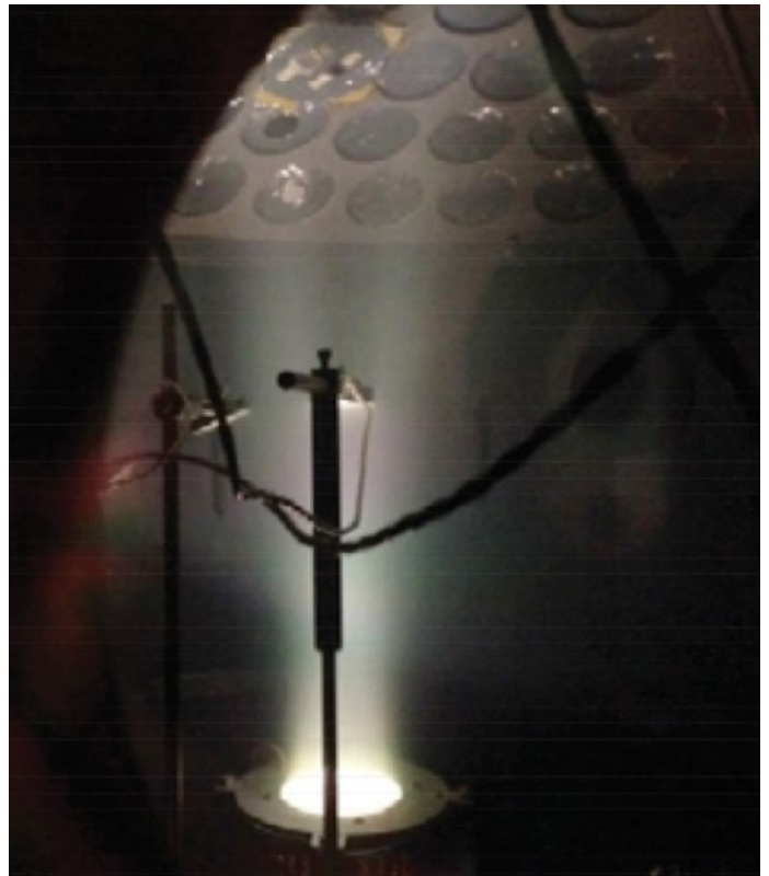
Figure 1: Denton Vacuum proprietary filament-free ion beam source.
