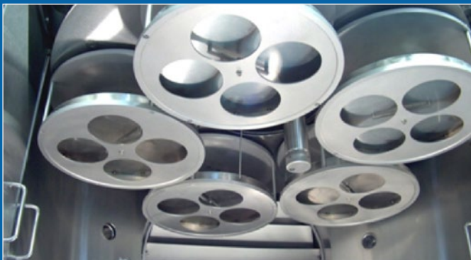
Multi-planetary Wafer Handling Fixture for High Uniformity, Multi-source Evaporation
